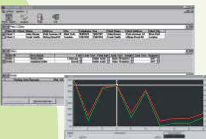
UniGas 3000+ XL can store 250 readings structured by boilers and customers. Using the optional **DBGas 2004** Windows™ software package, you can organize and manage your inspection and maintenance activity.
