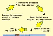
The MicroCal 20 is a documenting calibrator able to load test strategies using the CalPMan 2007 software. It can run them and store the results automatically, calculate the errors, highlight the out of range points, and download data on a PC to store them and to generate different reports. The calibrator internal memory can store a whole week procedures.
