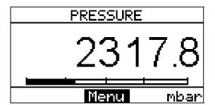
With the display filter activated, wait until the transient effect finishes (approx. 5 s).
