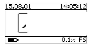
After switch-on, the MICROCAL P4 switches to the last operational mode used, e.g.:
